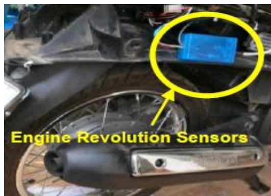
Fig. 7 The speed of engine unit from the Capacitor Discharge Ignition (CDI)
