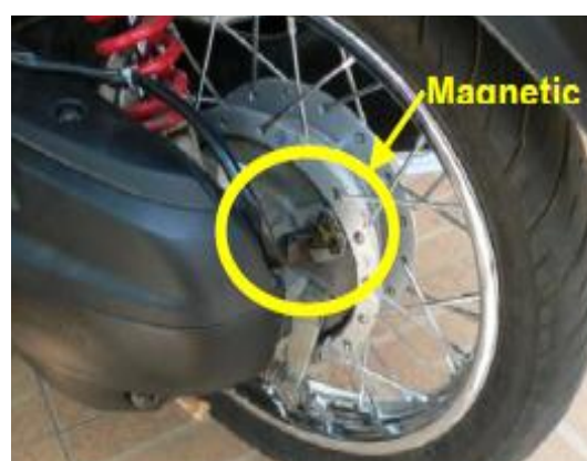
Fig. 6 The sensor on the rear wheel of the motorcycle.
